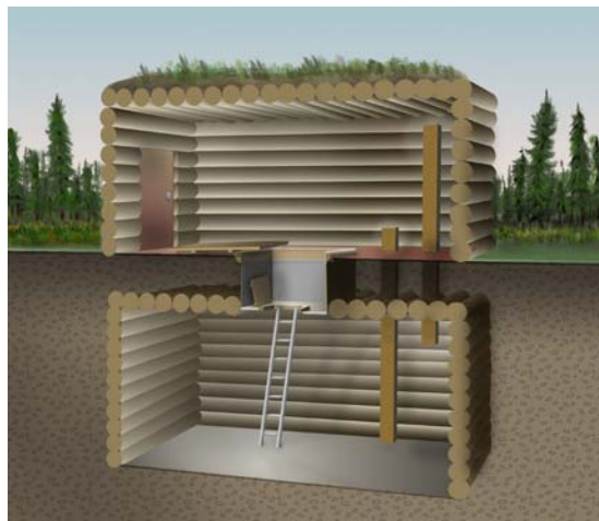
Figure 4. Soviet era deep cellar. Cellars are used for industrial purposes today or sometimes for an entire community
